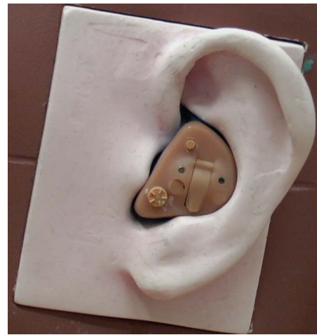
FIG. 2. (Color online) The left in-the-ear hearing aid with four different microphone directionalities.
