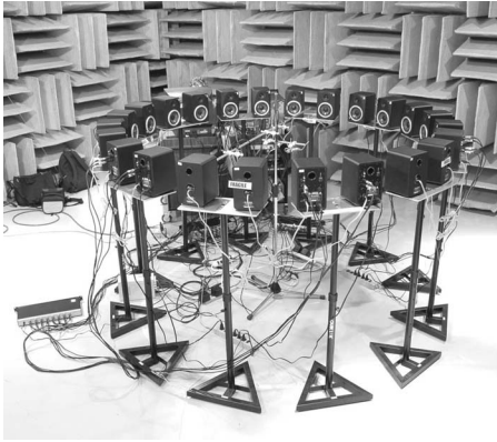
FIG. 4. Experimental AWFS setup in the hemianechoic chamber.
